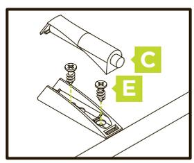
Mechanism should be placed flush with the front of rail/shelf as shown above. Mark and Pre-drill before installing.
