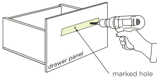
It is recommended to place a strip of masking tape across any area where you will be marking the door or drawer so that it can be easily removed if you make a mistake.
